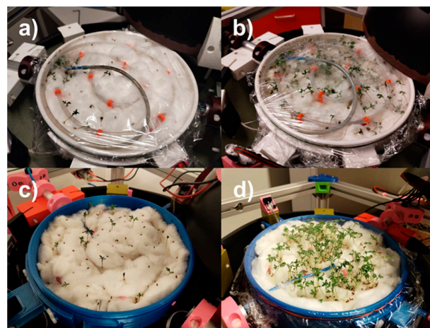
Figure 14. Results of Lepidium sativum L. cultivations: (a) cultivation in the clinostat with humidity 35% and light 10% of its maximum value, (b) cultivation in the clinostat with humidity 75% and light 8% of its maximum value; the static cultivation results (c) and (d) corresponding to the conditions of (a) and (b), respectively.
