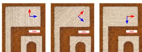
**Figure 5:** Detailed view of the top left area of three differently oriented (during printing) meander structures (left: 0°, middle: 45°, right: 90°)
