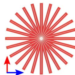
**Figure 6:** Star shaped structure with radial conductors (length of each radial conductor: 75 mm (midpoint to tip))
