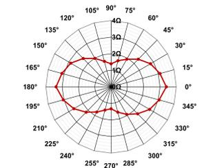
**Figure 7:** Resistances of radial conductors (median of 3 measurements) plotted against angle
