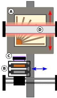
**Figure 1:** Top view of the setup within the printer and its basic components. A: Printing tray with substrate and printed object, B: Assembly with two print heads, C: UV light source, D: IR light source, red arrows: moving direction of the printing tray, blue arrows: moving direction of print head assembly
