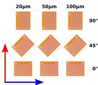
**Figure 4:** Array of meander structures with different layer thicknesses and angles of orientation with regard to the printing direction
