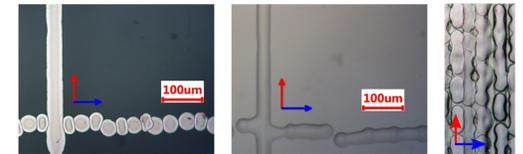
**Figure 3:** Printed drops on glass surface. left: silver ink, middle: non conductive ink (one layer), right: silver ink (multiple layers)
