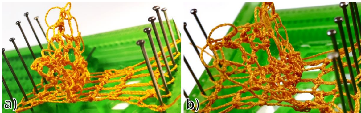
Figure 148. Photos of an SC textile in the shape of a T-beam made by repositioning within the CroMat prototype in the view from two sides (a) and b)).
