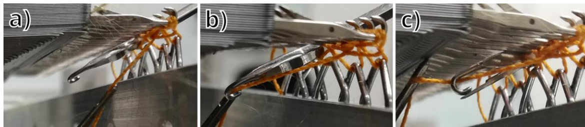
Figure 83. Movement of the yarn guide for the first variation of yarn over with a crochet needle inserted into the working stitch. a) Starting position of yarn guide and crochet needle. b) Moving the yarn guide in crochet direction with slightly changing the angle (T-axis) to place the yarn into the hook. c) Further change of angle with slight extension along Z and subsequent small movement against crochet direction to press the yarn securely into the hook. Crochet needle has changed its angle along W, closed the hook with the slider and begins to retract.
