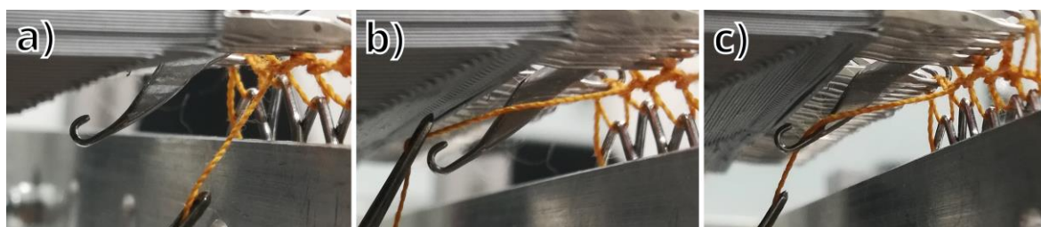
Figure 84. Movement of the yarn guide for the third variant of the yarn over using the example of a SC. a) Initial situation. b) Yarn guide changes angle and extends slightly to move closely over the open hook of the crochet needle and guide the yarn over it. c) Yarn guide retracts and moves slightly against crochet direction to push yarn into hook.
