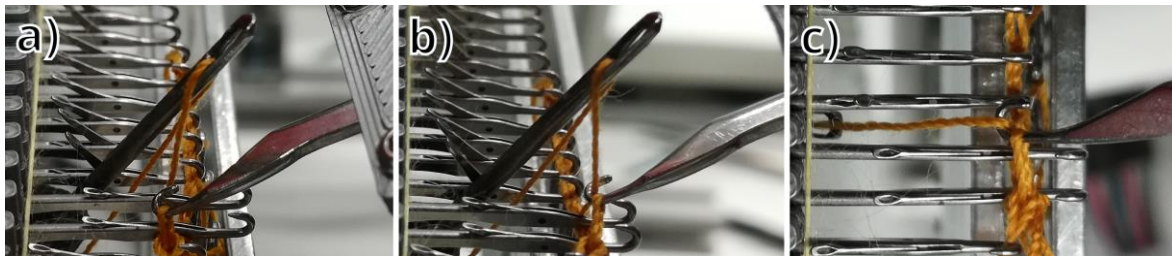
Figure 80. Fifth yarn over variant of the CroMat with the yarn guide being extended behind the crocheted textile. a) The crochet needle, which is in the position for laying over the LL of the last stitch, is moved towards the presented yarn segment. b) The hook catches and pulls the presented yarn segment. c) With the retraction of the yarn guide, the new loop is placed securely in the crochet needle's hook. Also, the LL is laid over the ANP.
