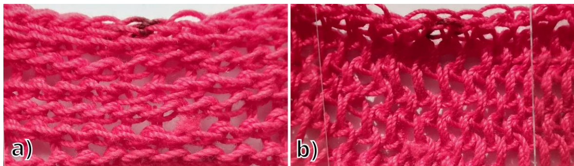
Figure 18. Photographs of fabrics consisting of SLs crocheted using the initial crochet machine prototype with manually moved machine elements. a) Technical face of the fabric. b) Technical back.
