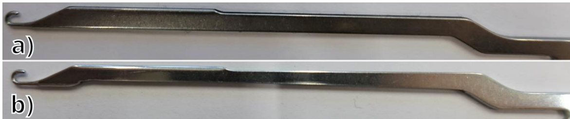
Figure 74. Modification of the crochet needle by grinding off approx. 1 mm on the underside in the area of the higher needle thickness. a) Original compound needle (SN-N 115.118 with slider SN-S 103.75 G1). b) Modified crochet needle.
