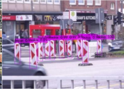
Fig. 5: Detector for construction-site beacons [GWH23]
