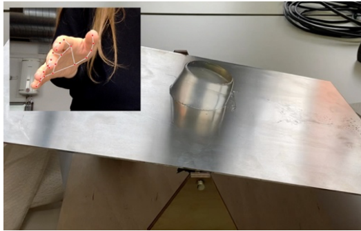
Fig. 3: Marina Köstel's project combines semisolid materiality, physical computing, and machine learning. Using Mediapipe's Handpose model, an interface tracks the y-axis position of the hand. The servo motor that controls the plate is adjusted according to the angle of the user's hand to ensure that the gelatinous material remains in balance. ©Ivan Iovine
