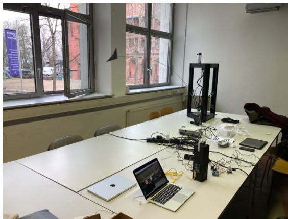
Fig. 2: Malte Niels Möllers' work, "Handling with Care", involves an interface that uses Mediapipe's Handpose model to track the acceleration of the wrist landmark on the x-axis. This parameter is used to control a stepper motor, which flies a small kite. ©Ivan Iovine
