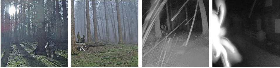
(a) A bright day with back-light. The camera needs a high dynamic range to be able to offer good images. (b) Foggy weather. The range of visual images is limited. (c) rain and snow in combination with (infrared) light blind the camera and thus also reduce the range. (d) Animals like spiders can also affect the range of the camera.
