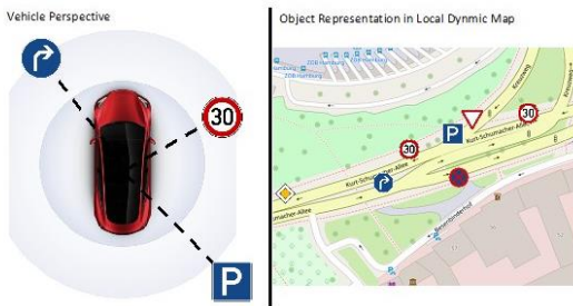
Fig. 10: Basic functionality for landmark-based localization [We23]
