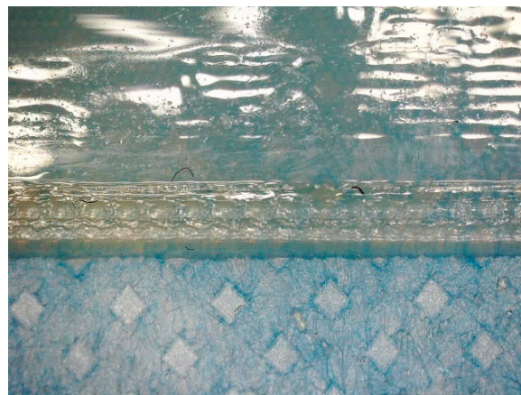
Figure 3. Fullcure720 (shiny area at the top) printed on a raft from Fullcure705 (visible in the middle as the border of the raft), printed on a PP nonwoven (blue part at the bottom). The long image size corresponds to 1.25 mm.
