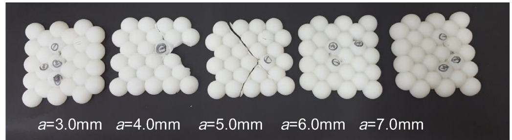
Figure 6. Stab resistant test results of samples with increasingly steeper egg-shell cores (from left to right). Reprinted from [50], Copyright (2018), with permission from Elsevier.
