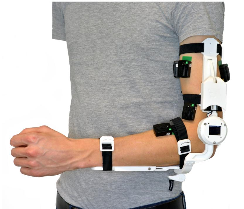
Figure 2: **Passive measurement orthosis and sEMG sensors used for simultaneous recording of elbow joint angle and muscle activation.** The measurement orthosis is mounted to the arm using flexible straps. The mounting points and the overall length of the orthosis is customizable to fit different arm geometries. The sEMG sensors are placed onto the *long* head and *short* head of the *biceps* and onto the *long* and the *lateral* head of the *triceps*. The wrist rotation is in neutral position.
