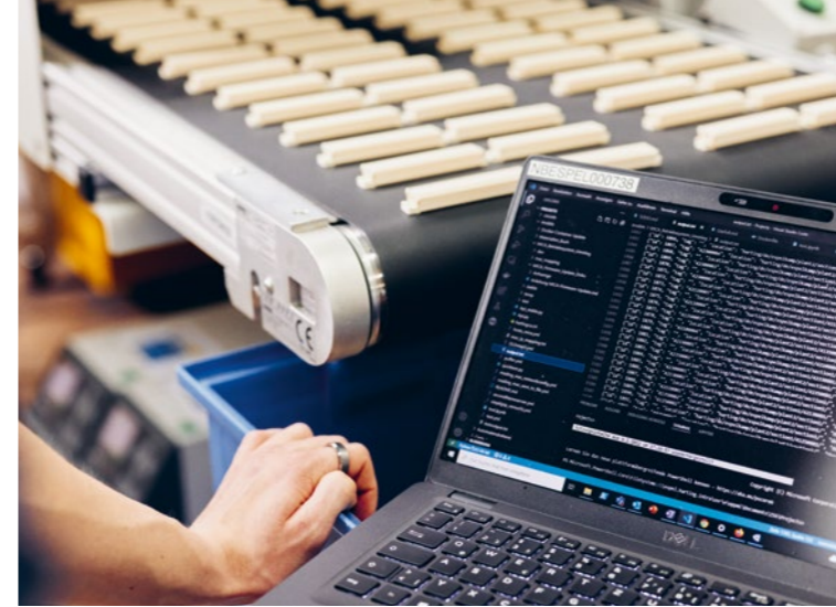
↳ Innumerable quantities of data, most of which is unstructured, are sent to the IIoT division each day. Electricity, compressed air and temperature are constantly monitored for each machine, including this one, which manufactures aluminium housing for industrial connectors
