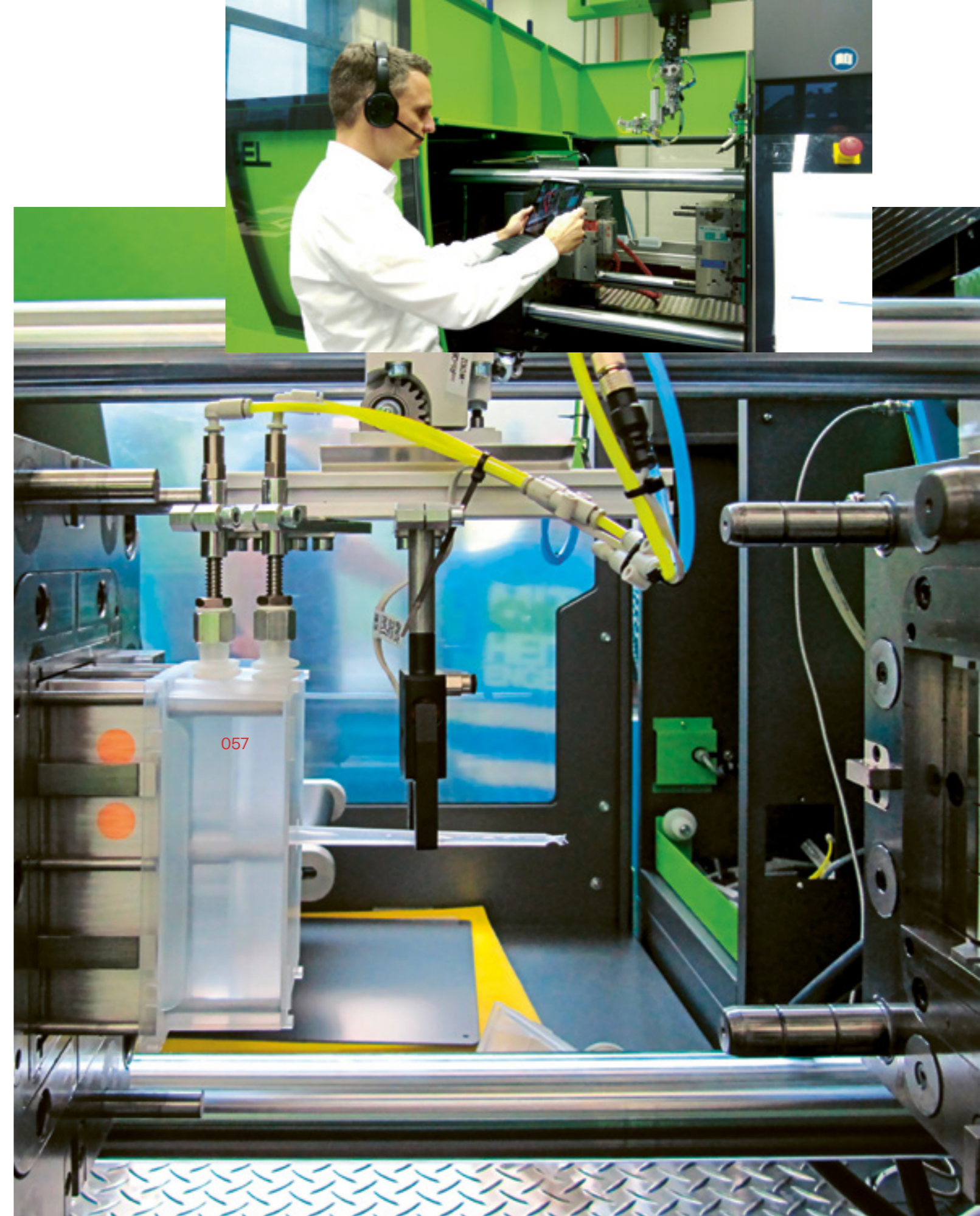
Automated production of a stack box: Thanks to a tablet camera supported by mobile wireless LAN, the students look into the injection moulding machine and give instructions on the system control.
